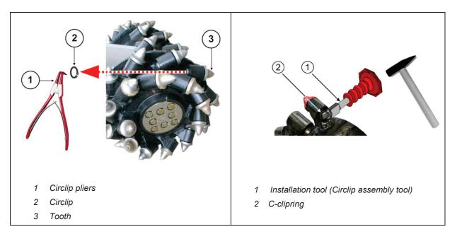
• Using a **hammer** and the **driver** or the **pin punch** and knock out the tooth from the tooth holder.
