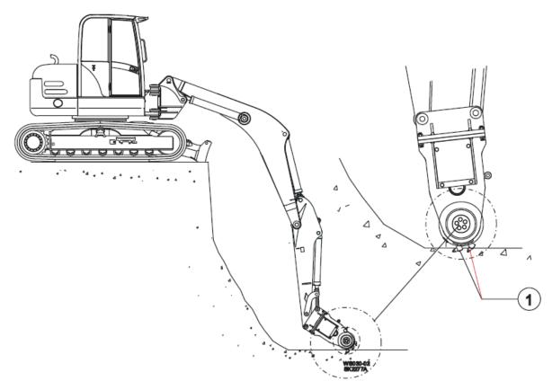
• Central bracket with static teeth allowing central (uncut) area to be excavated
