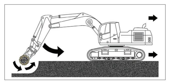
Cutting operations are best if the cutting unit drum moves into the direction of the attachment carrier. If the unit is moved sideways to achieve a larger cutting area, it must be ensured that the pressure on the excavator's boom, arm and cutting drum bearing is not too strong.
